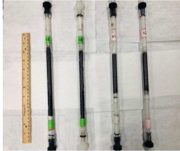
Figure 2-1. Photographs of packed-bed columns. The left-side photo shows lab-scale RSSCT setup including a feedwater tank, inline filter, peristaltic pumps, mixing jug, stirrer, syringe pump, and glass columns filled with GAC. The right-side photo shows glass columns filled with GAC in a packed-bed set using plungers and glass wool.
